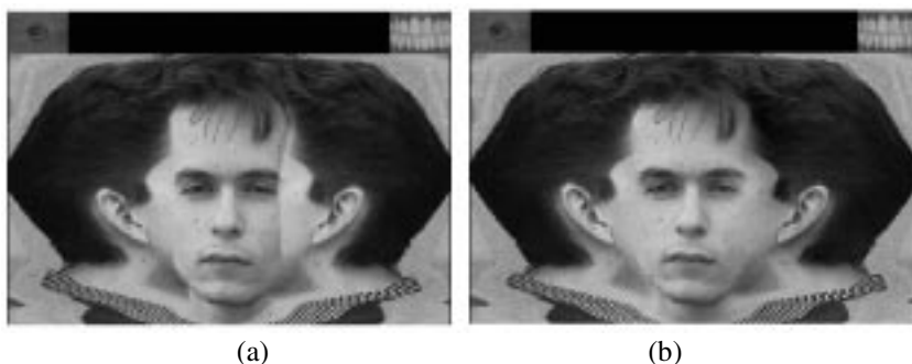
Fig. 3. Combining the texture images generated from the three (front, right and left) images without multiresolution techniques, in (a) and with the technique in (b).
